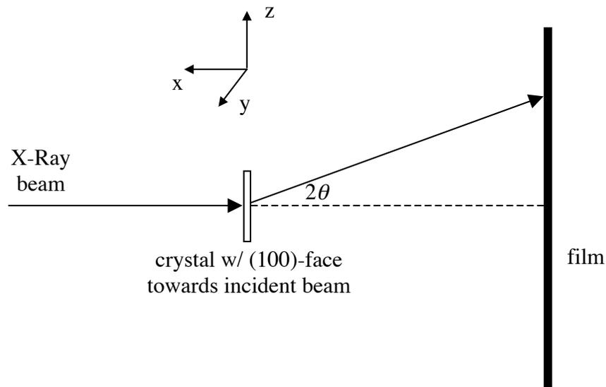
Scattering geometry for transmission Laue experiment.
